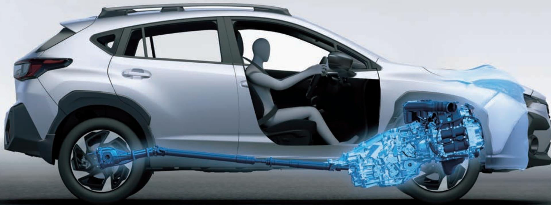
Designated crumple zones direct impact energy away from the ring-shaped passenger safety cell, while the Boxer engine is designed to slide below the cabin in a severe frontal collision.
