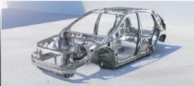
The Subaru Global Platform and ring-shaped passenger safety cell absorb and direct impact force around the cabin, rather than through it.
